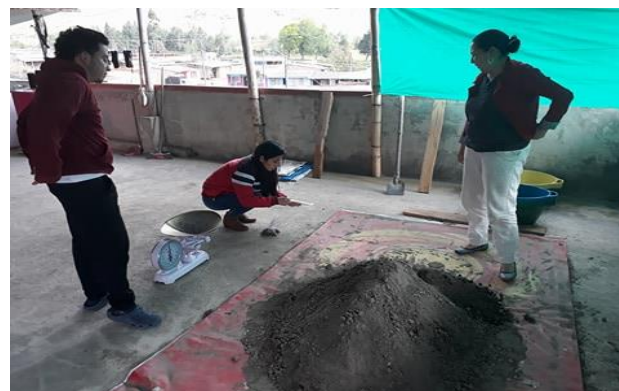
Figure 3 Contaminated sediments in the drying bed
