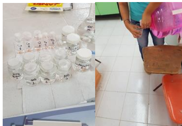
Figure 5 standard preparations for determination of NO 3 and Cobalt by the UV method
