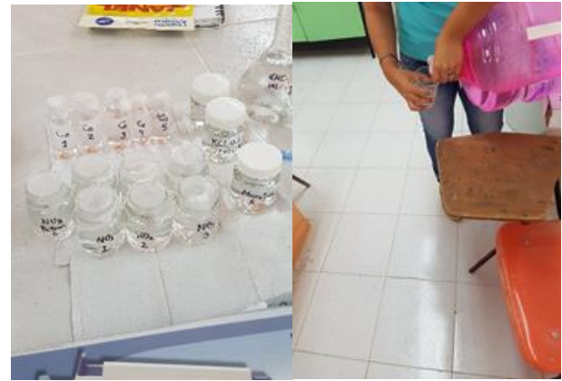
Figure 5 standard preparations for determination of NO 3 and Cobalt by the UV method
