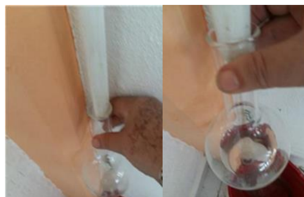
Figure 4 sample taking of condensed water from air conditioning Source: Own Elaboration
