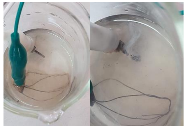
Figure 10 Electro plated silver nitrate solution Source: Own Elaboration
