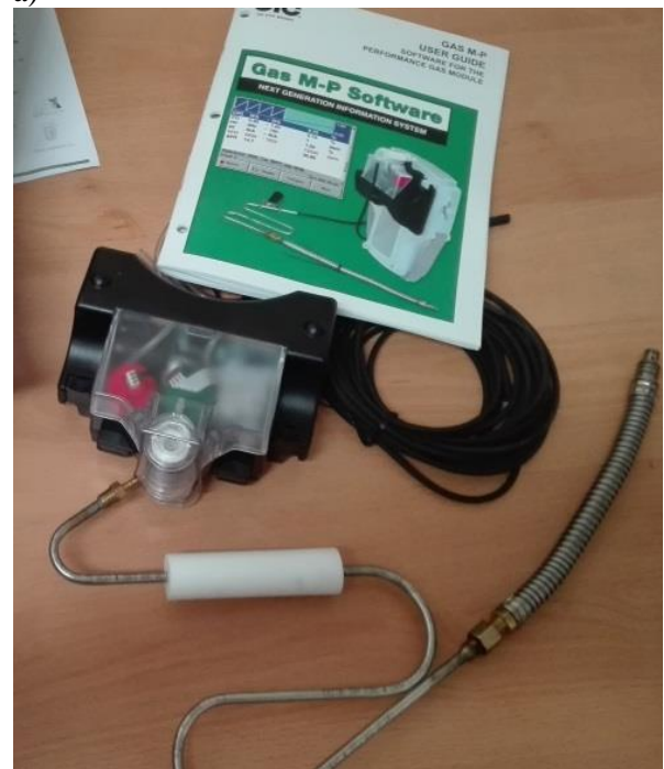
Figure 2 Pollutant gas measurement system a) Genesys NGIS Automotive Scanner b) M-P Gas Analysis Module Source: Own Elaboration
