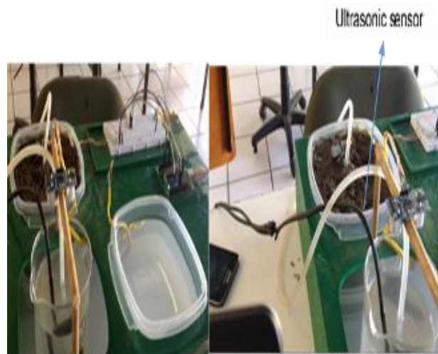
Figure 1 Model of the irrigation system, the Ultrasonic sensor shown
