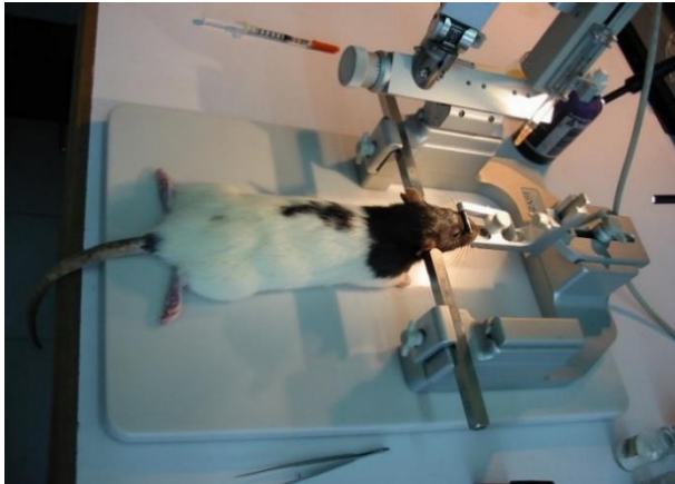
Figure 4 Mounting the animal on a standard stereotaxic device. The animal remains attached to the ear bars by the auditory meatus and the muzzle by the bar of the incisors
