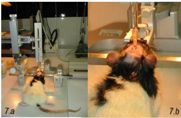
Figure 7. 7.a) Image showing the way in which the microinjection was performed by means of the nanomolar infusion pump mounted on the stereotactic apparatus. 7.b) The needle of the microinjector freely crosses the cerebral cortex and the thalamus of the animal until it reaches the anterior hypothalamus.
