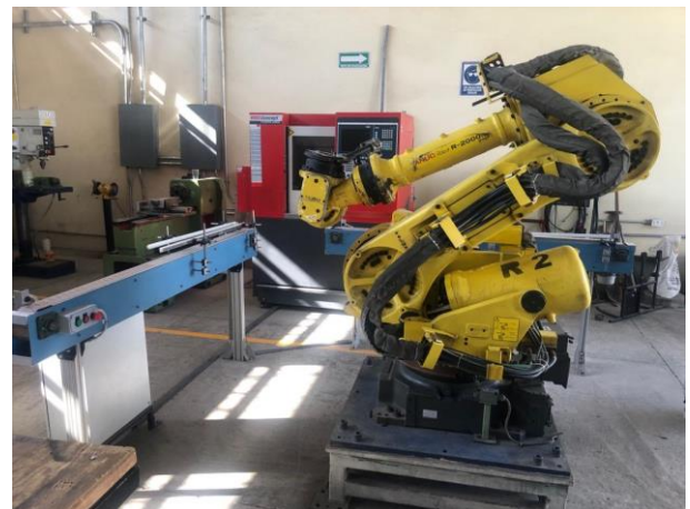
Figure 6 Lateral view of the reengineering applied to the manufacturing cell Source: Own elaboration
