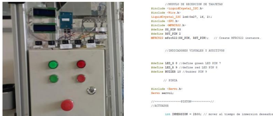
Figure 4.5 Control area of the final prototype and programming libraries
