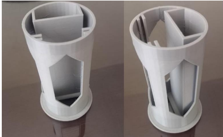
Figure 1.12 PLA container used for the structural subsystem
