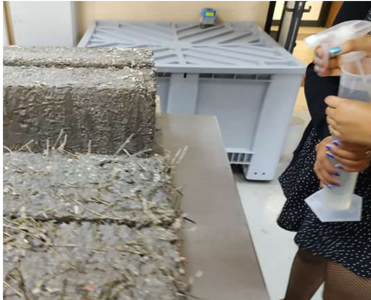
Figure 9 Application of water with a spray bottle for curing the ecoblocks
