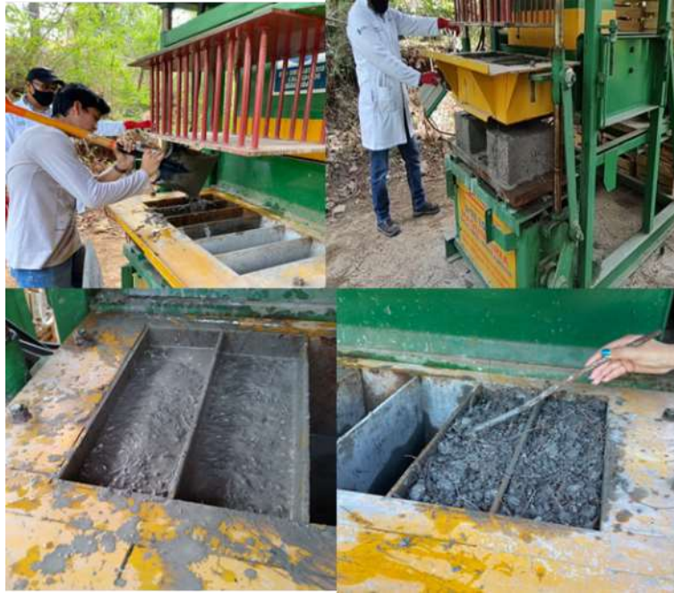
Figure 5 Production process of the two ecoblock prototypes in the vibroblock machine
