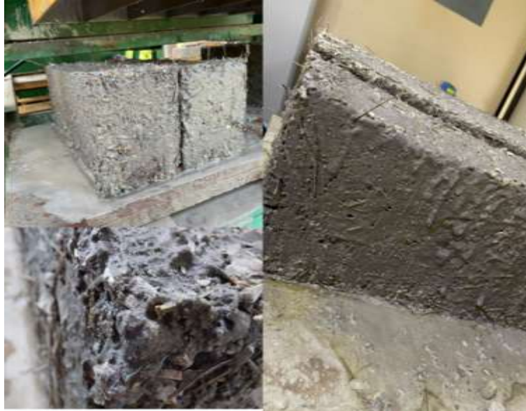
Figure 7 Ecoblock with ocoxal leaf bearing
