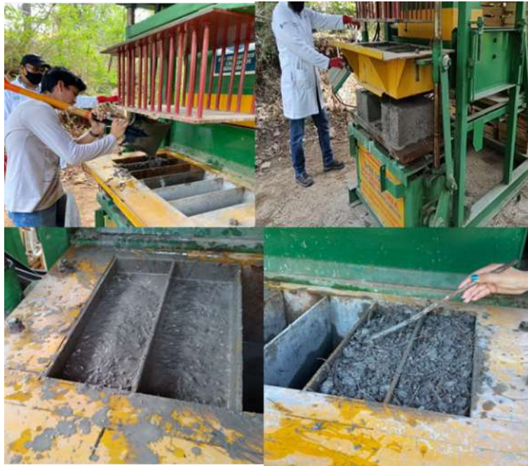
Figure 5 Production process of the two ecoblock prototypes in the vibroblock machine
