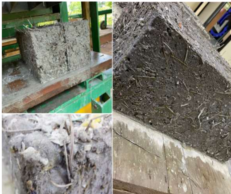
Figure 6. Ecoblock with ocoxal leaf bearing.
