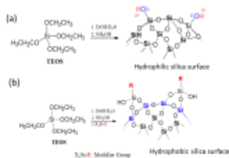
Figure 1. (a) Production of hydrophilic silica (b) Production of hydrophobic silica
