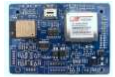
Figure 7 Final Result of Paste Application and Component Assembly
