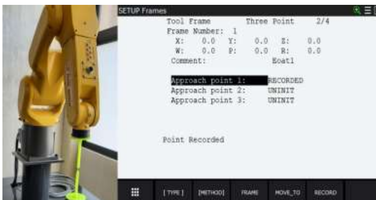
Figure 2.8 Step 1 of the three points method for declaring tools
