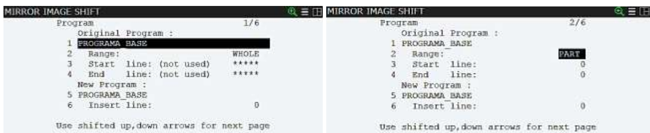
Figure 3.18 Program Shift screen, a) For a whole program b) For a part of a program
