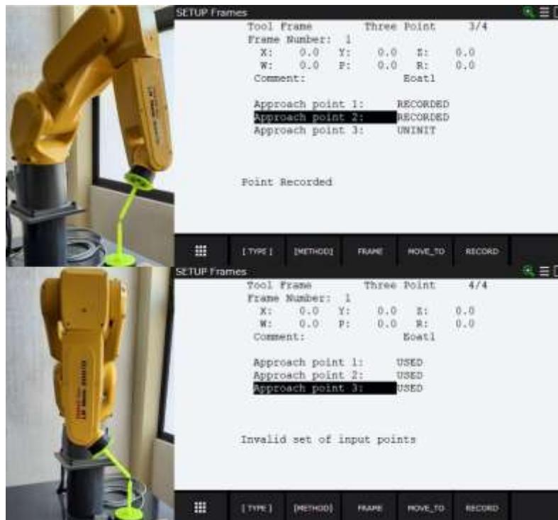
Figure 2.9 Step 2 and 3 of the three points method for declaring tools
