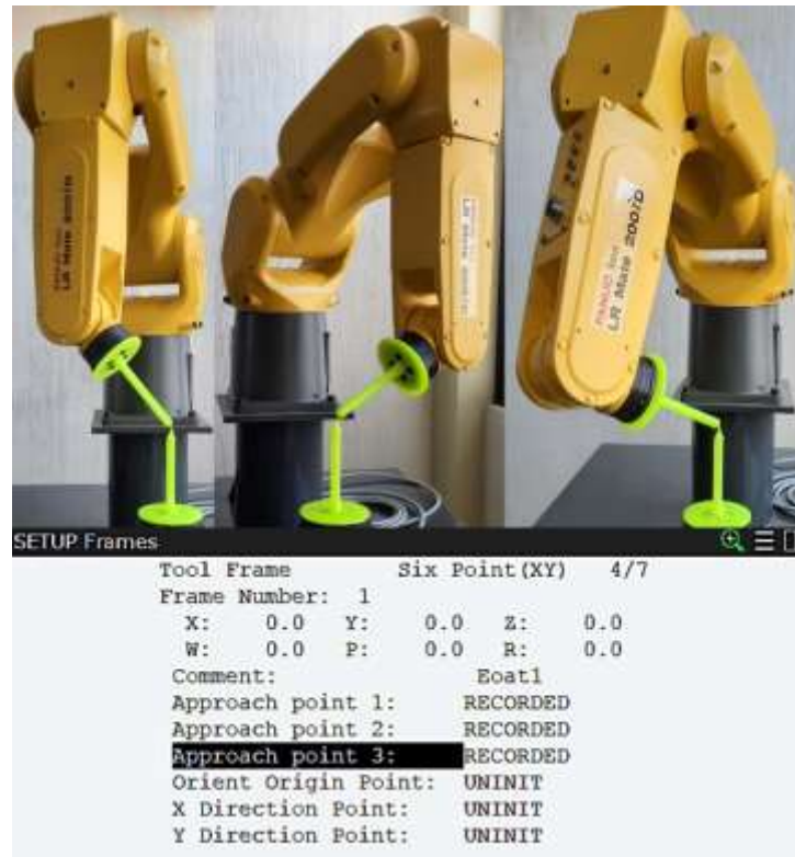
Figure 2.10 Step 1 of the six point method for declaring tools
