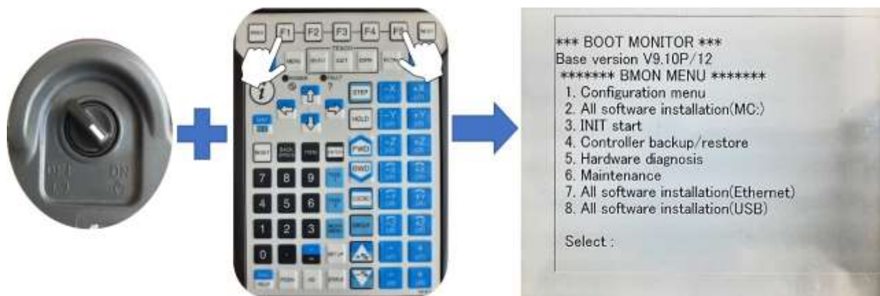
Figure 5.26 Startup to access the BOOT MONITOR memory
