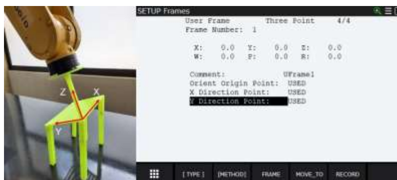
Figure 2.19 Step 4 of the three points method for declaring USER frames
