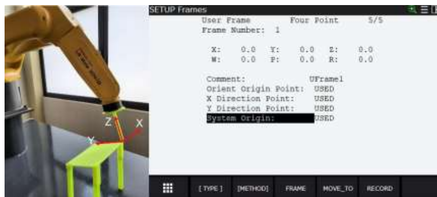
Figure 2.21 Step 2 of the four points method for declaring USER frames
