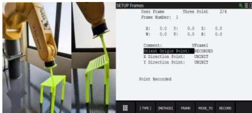
Figure 2.16 Step 1 of the three points method for declaring USER frames
