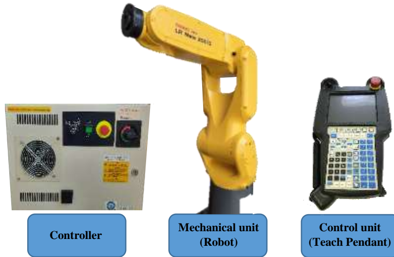
Figure 1.1 Main parts of the Fanuc LR Mate 200iD robot
