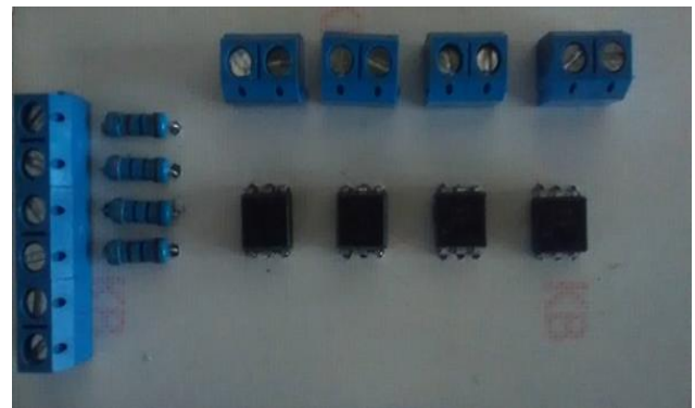
Figure 5 PCB of the opto-couplers circuit.
