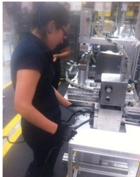
Figure 2.20 Operator inserting the conduit in the chamber
