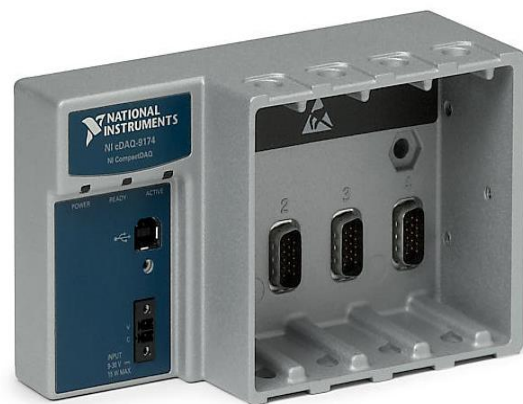
Figure 2.5 NI Cdaq-9174 chassis
