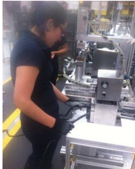
Figure 2.20 Operator inserting the conduit in the chamber
