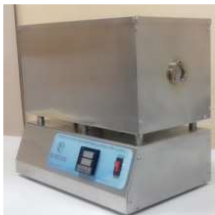
Figure 1.2 Horizontal Tube Resistive Furnace (CMOD-HAT-1100D25)
