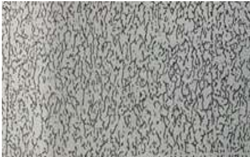
Fig. 20 Low carbon Steel to 100X. Grain 9. Metals Handbook
