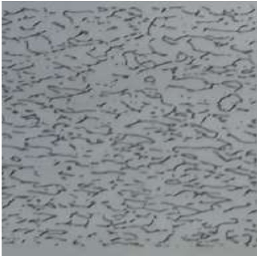
Figure 14 Steel 1008 a 250X, with 30% of reduction. Metals Handbook
