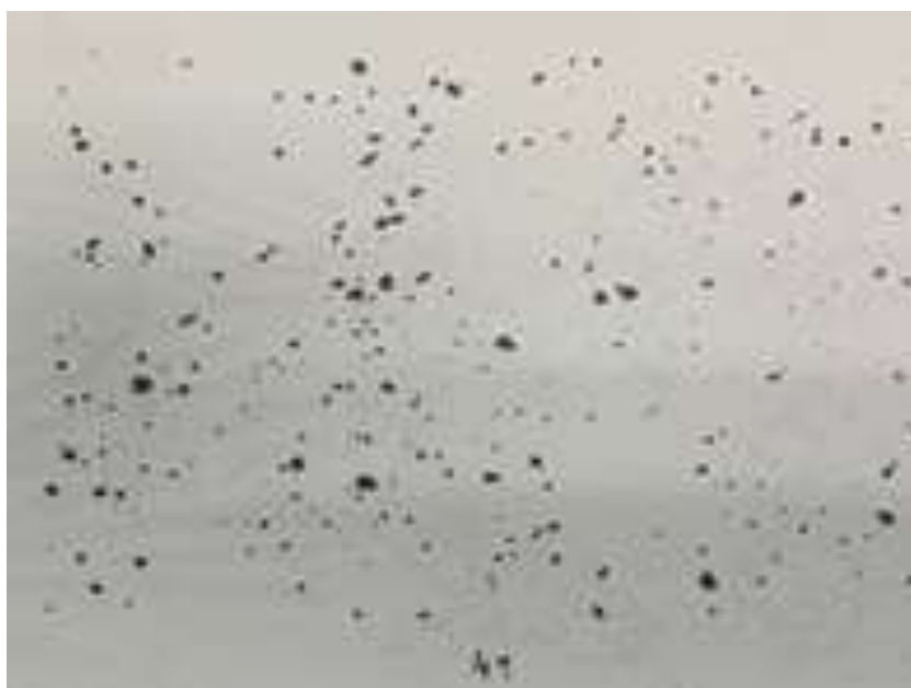
Figure. 23. Steel 12L14 without attack to 100X. It shows Comet tails resulting from directional polishing. Metals Handbook
