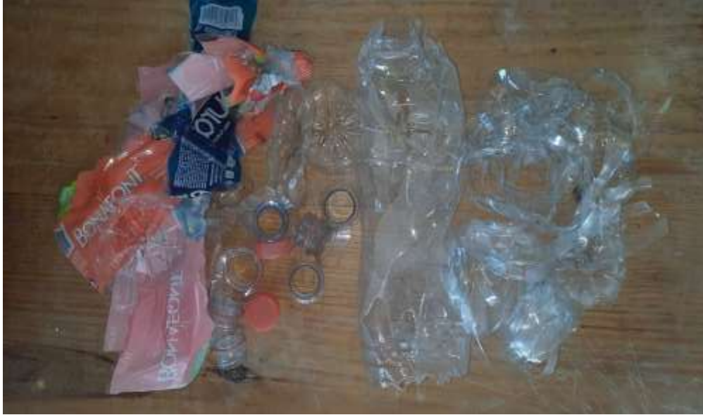
Figure 5 Removal of labels and caps from the collected bottles
