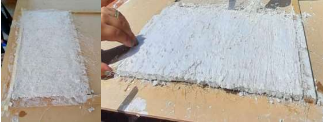
Figure 18 Placement of the Ixtle fibers in the pouring of the mixture on the wooden mold
