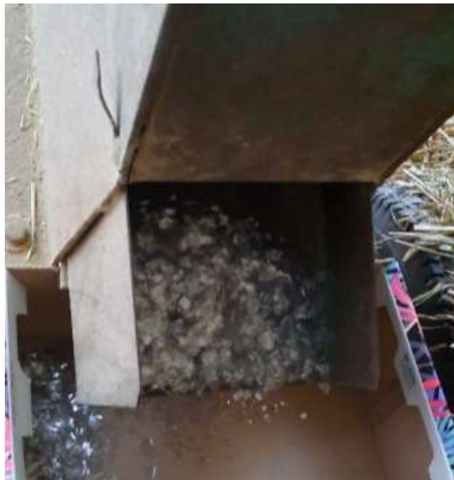
Figure 8 Obtaining plastic milling for panel use
