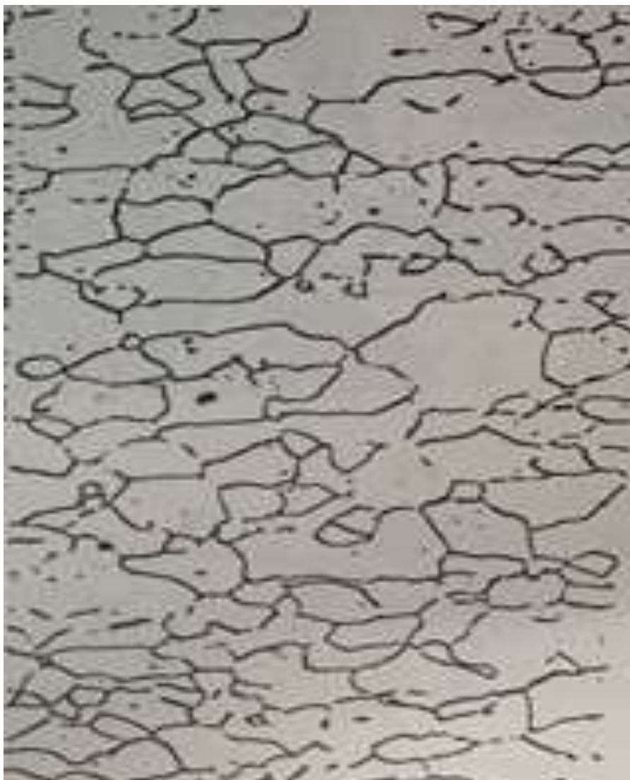
Figure 18 Low carbon Steel to 100X. Coarse ferrite. Grain 5. Metals Handbook
