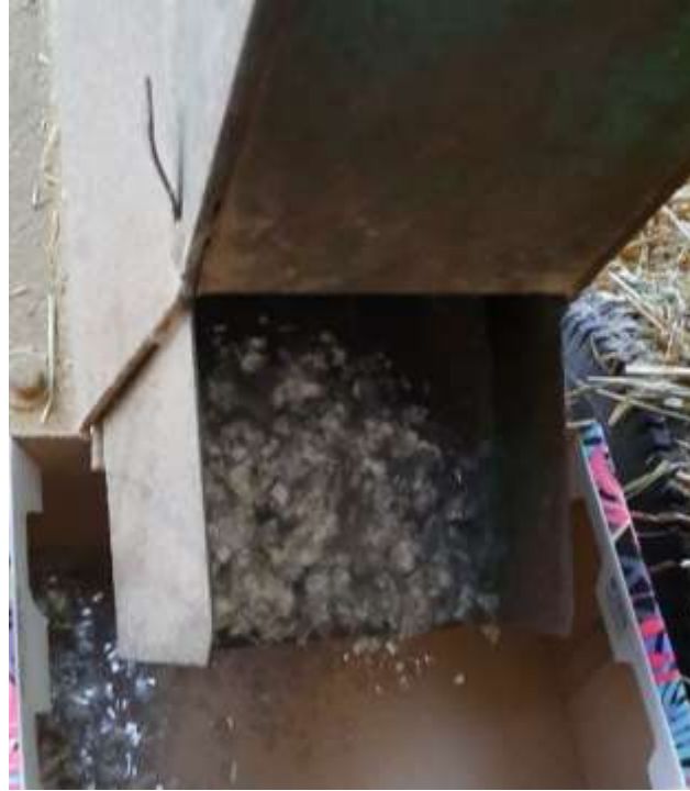
Figure 7 Expulsion through the output chamber of ground plastic
