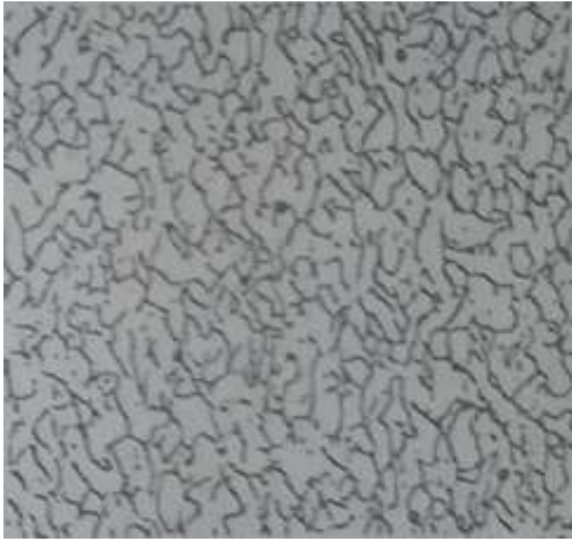
Figure 14 Steel 1008 a 250X, with 30% of reduction. Metals Handbook
