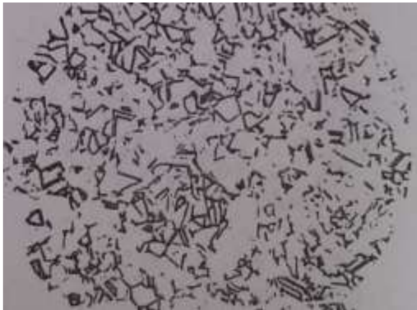
Figure. 22 Equiaxed grains. Brass 260 to 75X. Size of grain 0.035 mm annealing to 482°C. Metals Handbook
