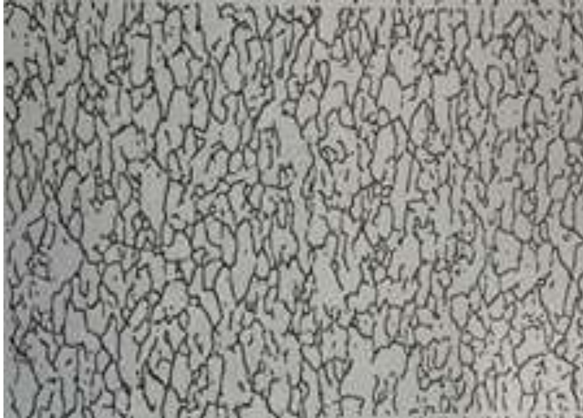
Fig. 20 Low carbon Steel to 100X. Grain 9. Metals Handbook
