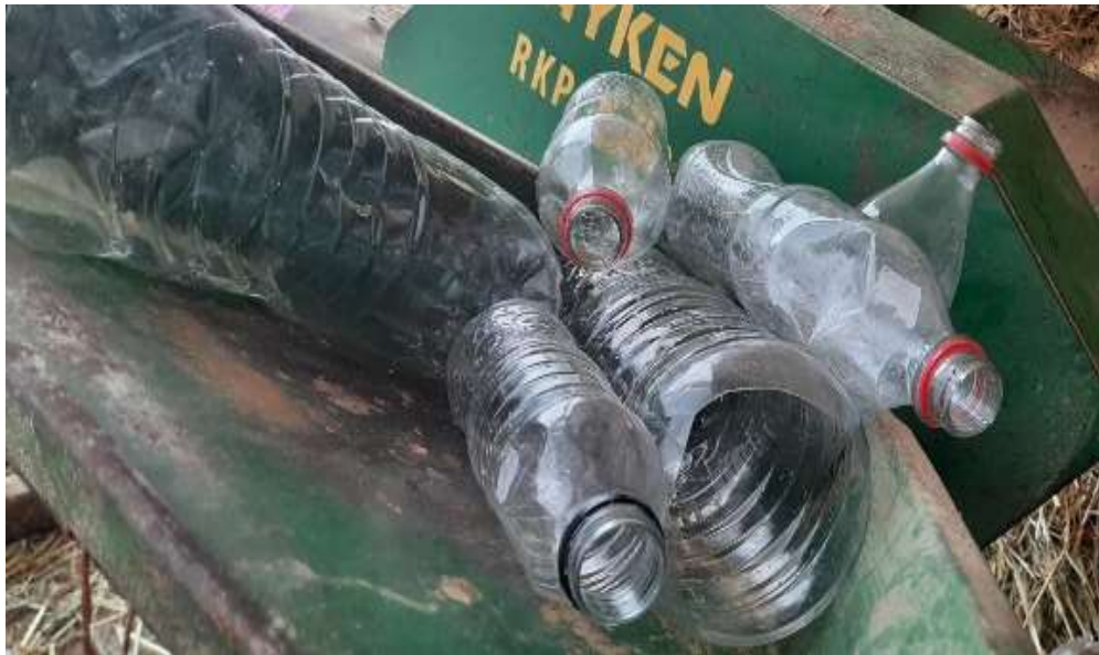
Figure 6 Entry of bottles to the hopper of the plastic materials mill
