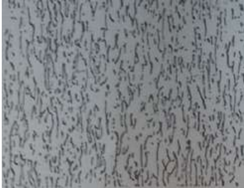
Figure 17 Steel 1008 to 250X, with 60% of reduction by cold rolled. Metals Handbook
