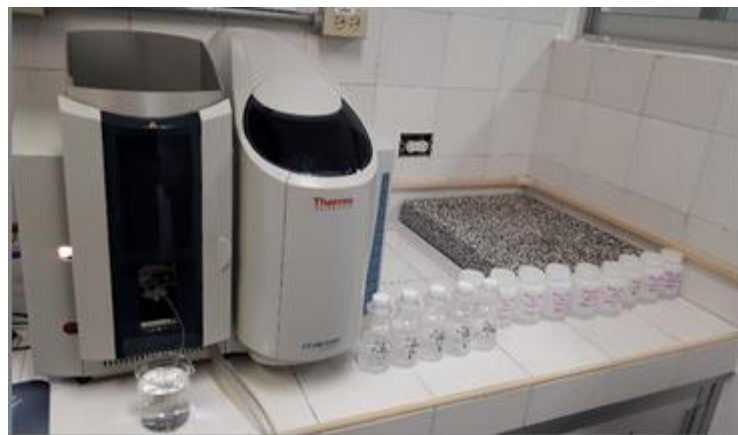
Figure 6.2 Atomic Absorption Spectrophotometer, Thermo Scientific Brand, model iCE 3000 Series AAS used in this work
