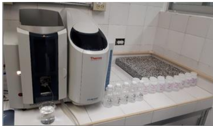
Figure 6.2 Atomic Absorption Spectrophotometer, Thermo Scientific Brand, model iCE 3000 Series AAS used in this work
