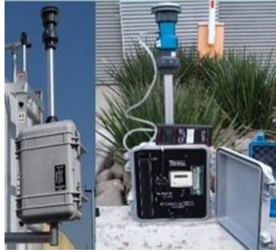
Figure 6.1 PM10 Sampling using the Minivol sampling device
