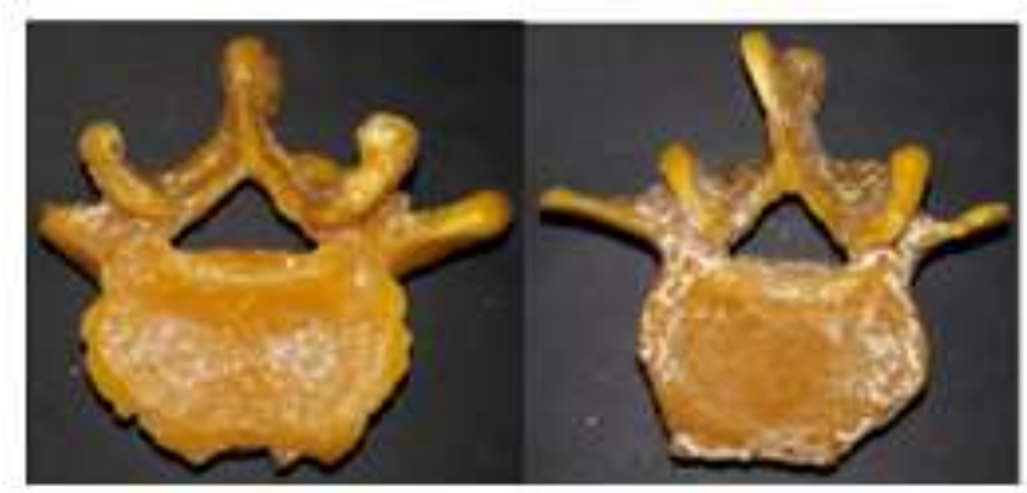
Figure 5.6 Plaster model with the lost wax technique.
