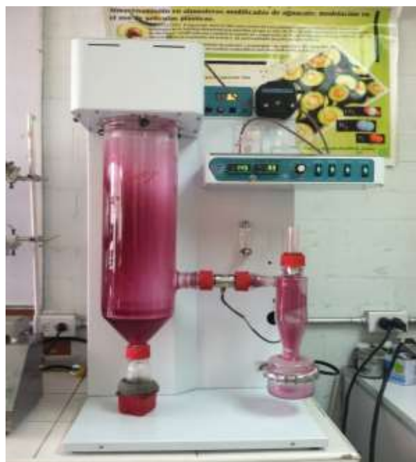
Figure 10.1 Microencapsulation by spray drying
