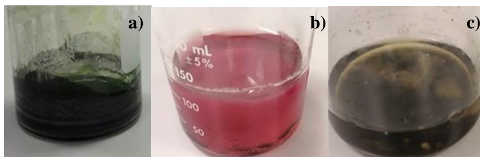
Figure 7.6 Image of the extract obtained by maceration process: a) without purification process, b) purification with hexanes and c) purification with hexanes and ethyl acetate
