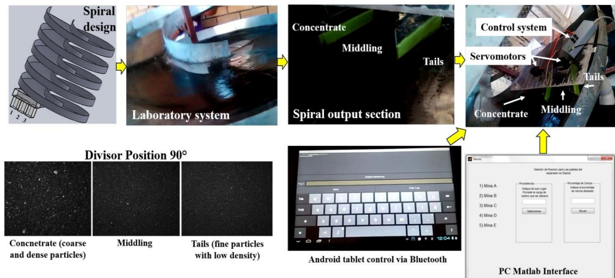
Figure 5.2. System of monitoring and control of the movement of splitters by direct and remote connection via Bluetooth (Ibid 145).
