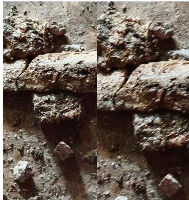
Figure 3.1 Solidified grease extracted from the drainage, causing obstruction and bad odors, this was due to the direct discharge of used vegetable cooking oil from a dwelling house into the sink
