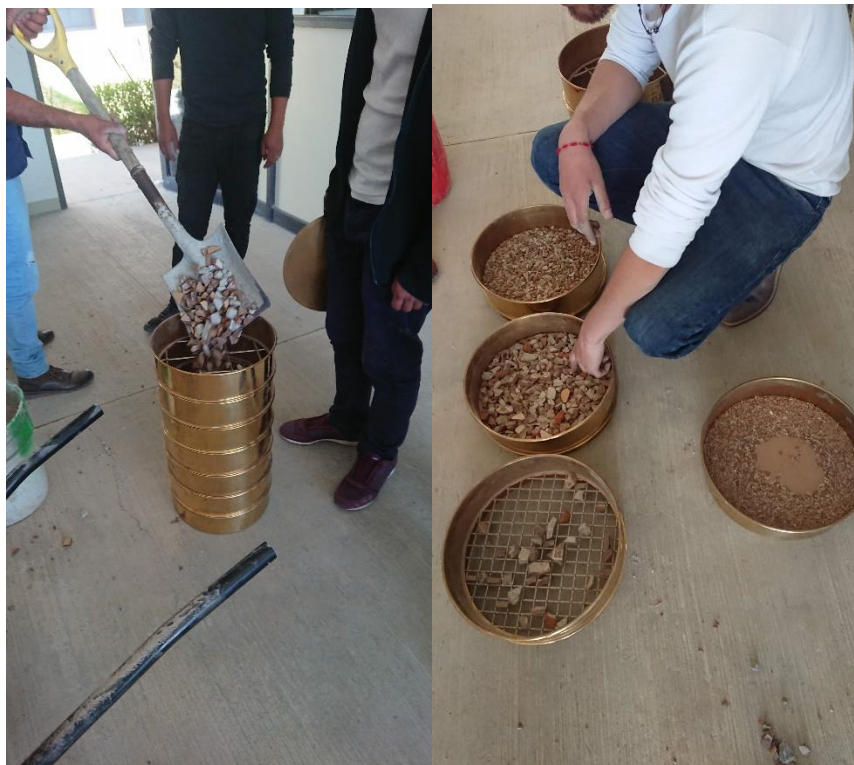
Figure 4.4 Screening of the material and particle size of the stone aggregate or aggregate
