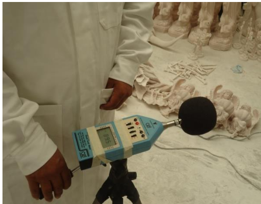
Figure 7.2 NSCEAT measurement with an integrating sound level meter in the resin pouring area
