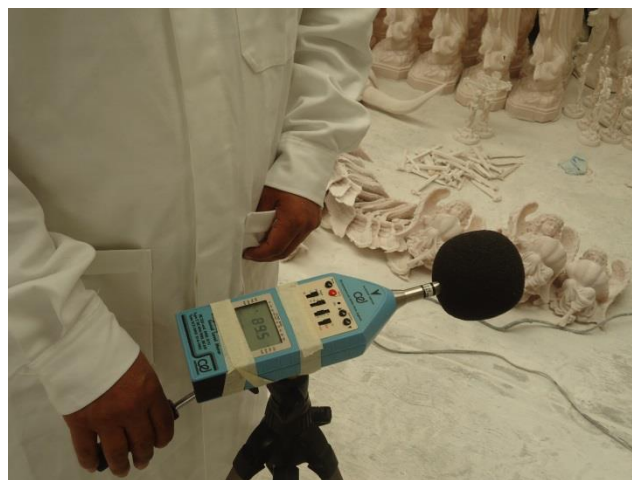
Figure 7.3 NSCEAT measurement with an integrating sound level meter in the resin pouring area
