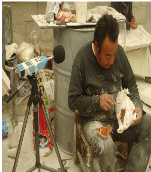
Figure 7.7 NSCEAT measurement with type 2 integrating sound level meter, in the patching area
