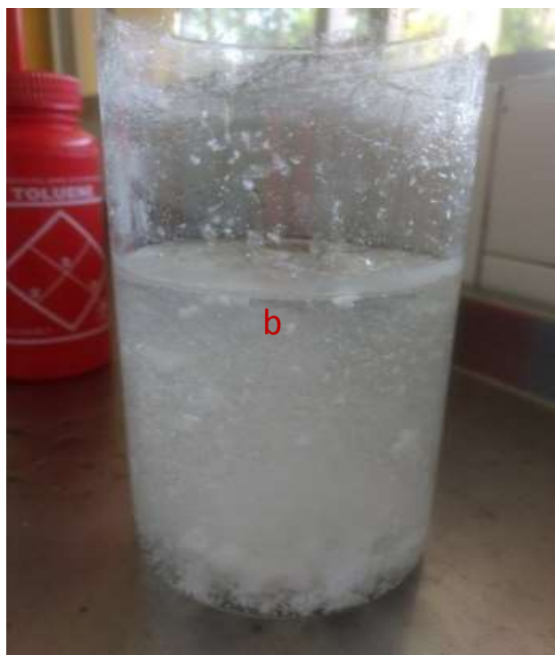
Figure 5 Washing and crystallization of the oligomer derived from Alkoxybenzoates and alkyl halides Own Source
