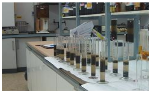
Figure 2 Tests of the optimum coagulant, as well as its optimum coagulant dosage
