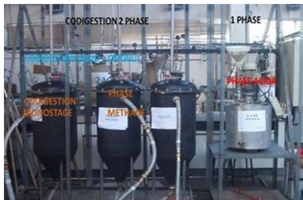
Figure 1 Phased co-digestion and single-stage co-digestion digesters
