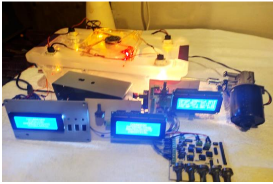
Figure 4 Prototype of the artificial incubator
