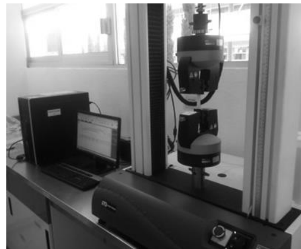
Figure 7 Tensile test in the biopolymers. Source: Own Elaboration
