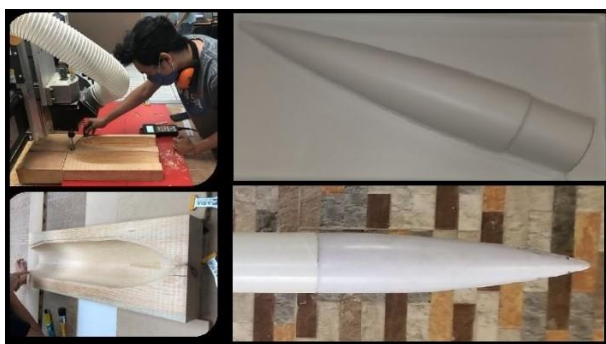
Figure 3 Rocket nosecone manufacturing process Source: Own elaboration
