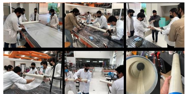
Figure 5 Rocket fuselage manufacturing process Source: Own elaboration
