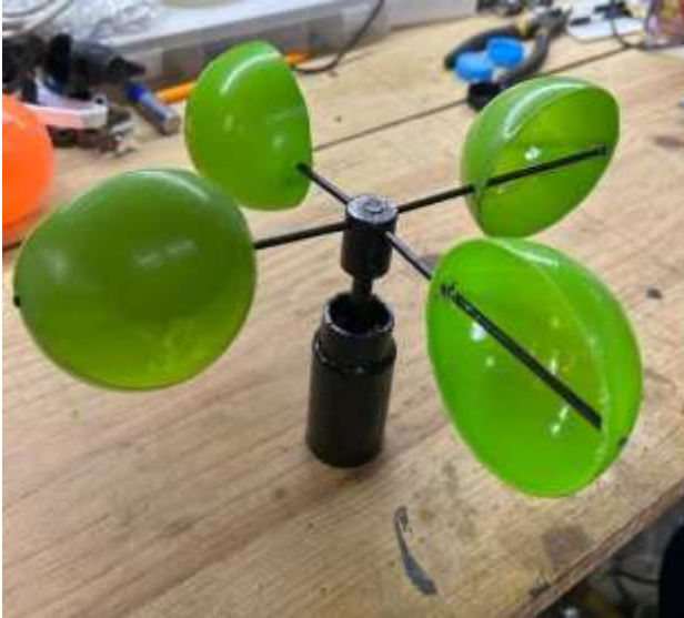
Figure 10 Prototype anemometer usable for testing (2023)
