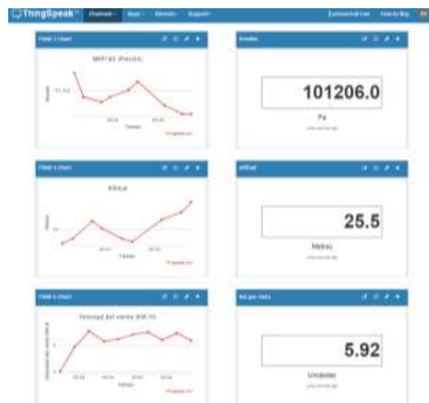
Figure 14 Sensor data collection on the ThingSpeak platform. Part 2
