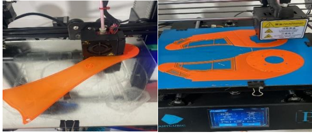
Figure 4 3D printing of the rotating column
