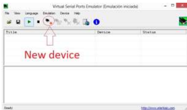
Figure 17 Creating a new device in the virtual serial port emulator VSPE
