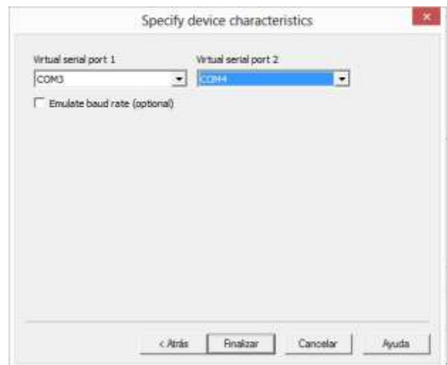
Figure 19 Selection of ports in VSPE to carry out emulation
