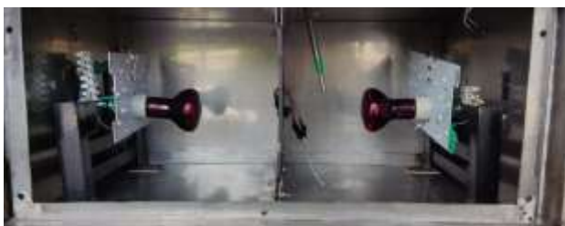
Figure 1 Plastic aging chamber with two infrared luminaires Source: Self Made
