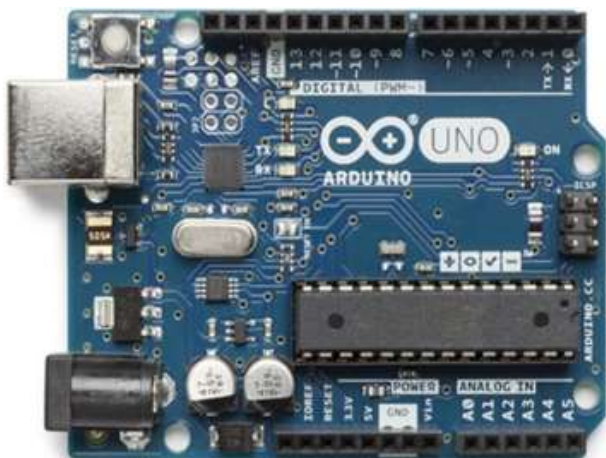
Figure 8 Arduino UNO board Source: https://arduino.cl , 2021
