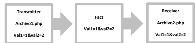
Figure 3 Parameter passing by PHP's GET method
