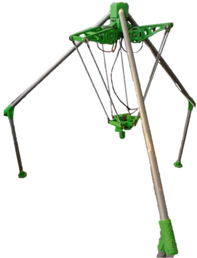
Figure 3 Delta parallel robot prototype used Source: Own elaboration, 2021
