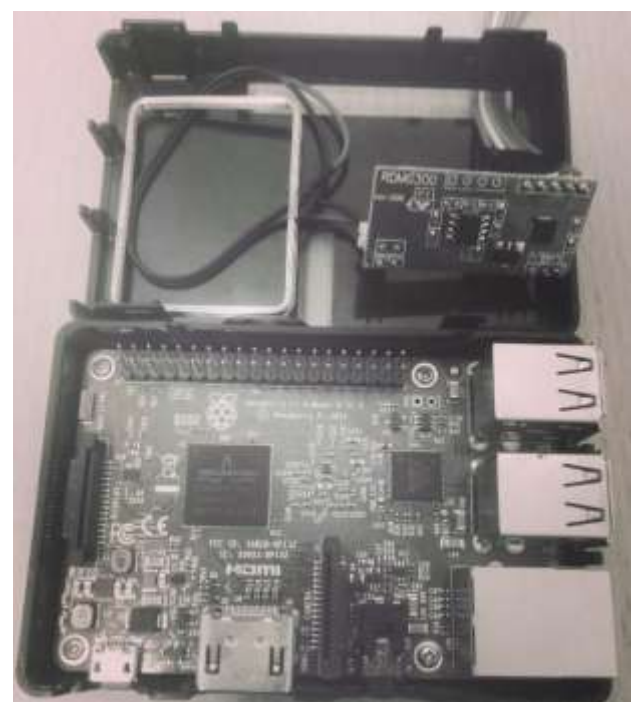
Figure 3 Raspberry Pi and RDM6300 sensor
