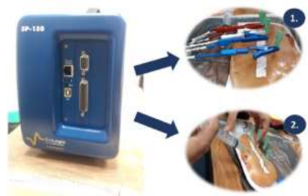
Figure 1 EIS device (left) connected to chicken breast at 1) basal stage and 2) after being injected with nanoparticles
