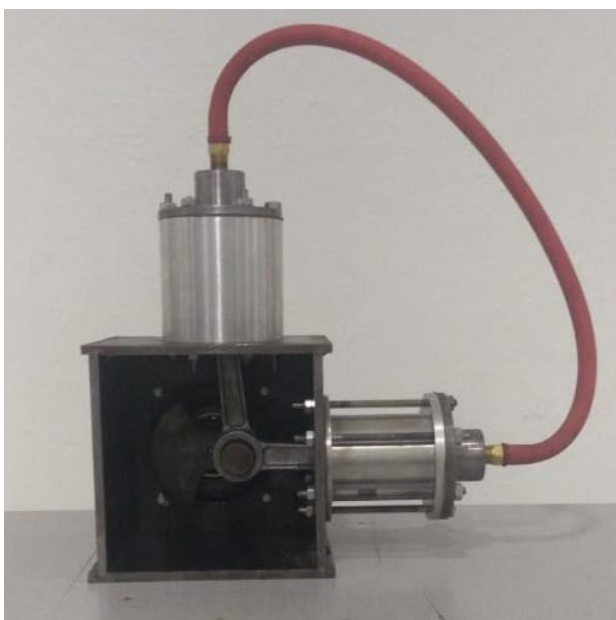
Figure 12 Finished prototype of a Stirling engine rear view
