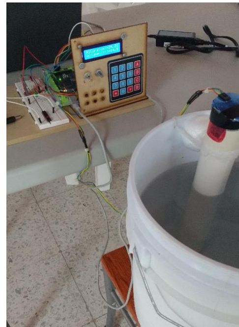
Figure 12 Integration of the elements for the water level measurement system contained in the bucket
