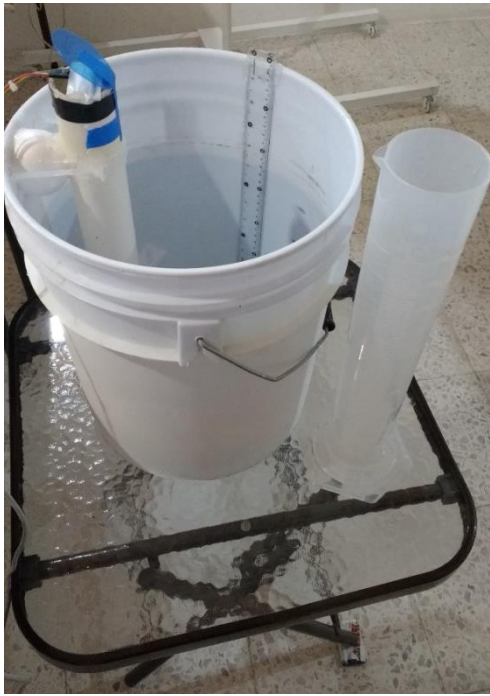
Figure 19 Container with terminal strip, PVC tube with ultrasonic sensor and graduated beaker Source: Own Elaboration
