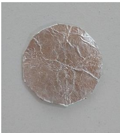
Figure 11 Disc type float, aluminum lined cork material placed in the PVC pipe
