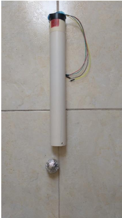
Figure 10 PVC tube assembly, ultrasonic sensor with cables and aluminum-lined unisel sphere.
