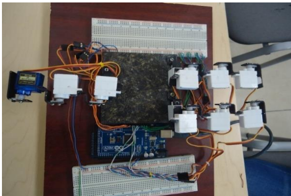
Figure 8 Manipulation system with \mathbf{q} = [0^\circ, 0^\circ, 0^\circ, 0^\circ] configuration for each robot petit.
