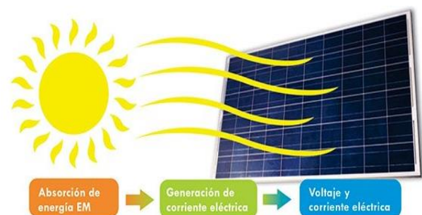
Figure 2 General view of how a solar cell work
