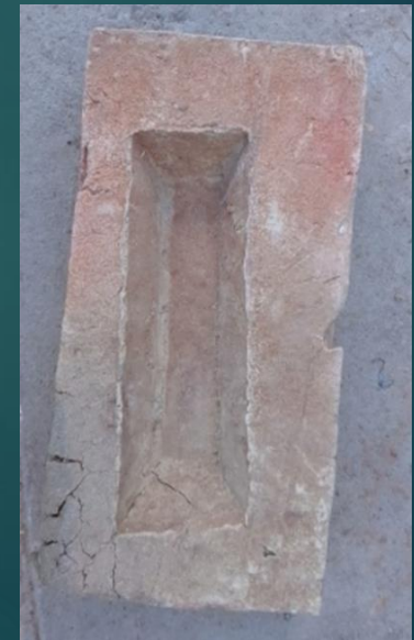
BRICK WITH BAD QUALITY
