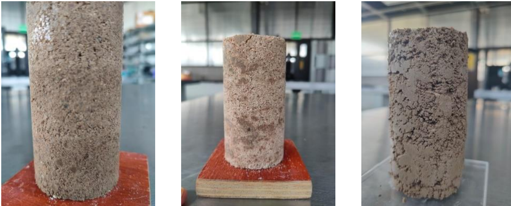
Figure 3. Left: MH1 with a 15% moisture content. Central: MH1 with a 20% moisture content. Right: MH1 with a 30% moisture content.
