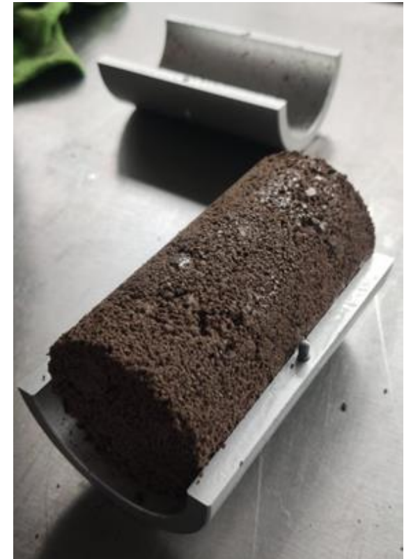
Figure 4. Soil sample after compaction in the used mold.
